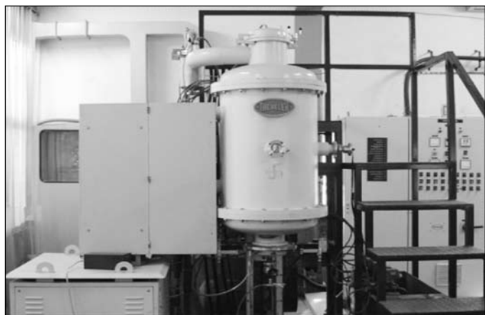
Fig. 3. Setup for chemical vapor infiltration
