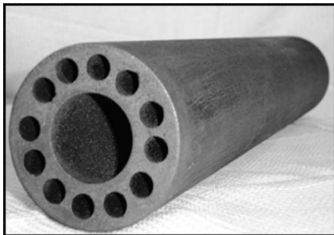
Fig. 1. Photograph of a channel tube fabricated with carbon-carbon composite
